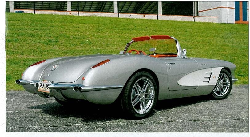
was done by Cory McDonald.) The original windshield side posts and door-pillar posts were restored and rechromed and all the stainless-steel trim on the windshield frame, doors and decklid was straightened by hand and polished to a brilliant shine.
