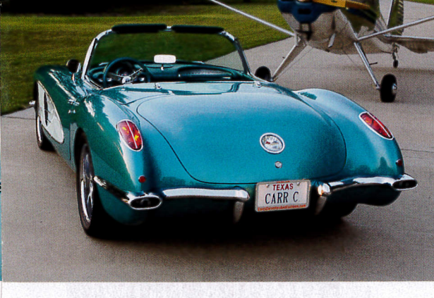
One look at the car in "as discovered" form (top left) and it's clear that this was no typical restomod project. Jettisoning the rusty stock frame for an Art Morrison setup provided a suitably modern foundation, to which builder Carr Campbell bolted a tweaked LS3, a five-speed trans and manhole-sized Wilwood brakes. A high-shine take on the original Crown Sapphire paint keeps the look firmly anchored in the '50s, even if the car's performance is more in line with that of a C7.
