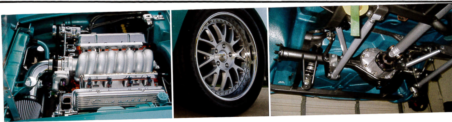
A dressed-up LS376 crate engine generates around 500 hp, while 18-inch rolling stock and a customized nine-inch rear end help deliver it to the ground.
