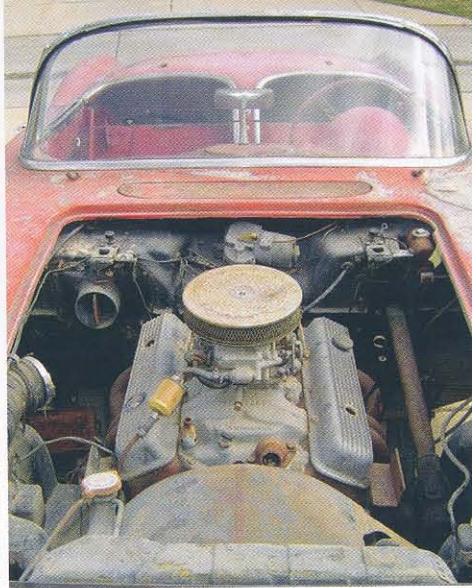
Counterclockwise from above: Non-original engine; accident-damaged exterior; missing trim; LT4 was stroked and fitted with various hot-rod parts, boosting power to 440 bhp; interior looks stock, but isn't.
